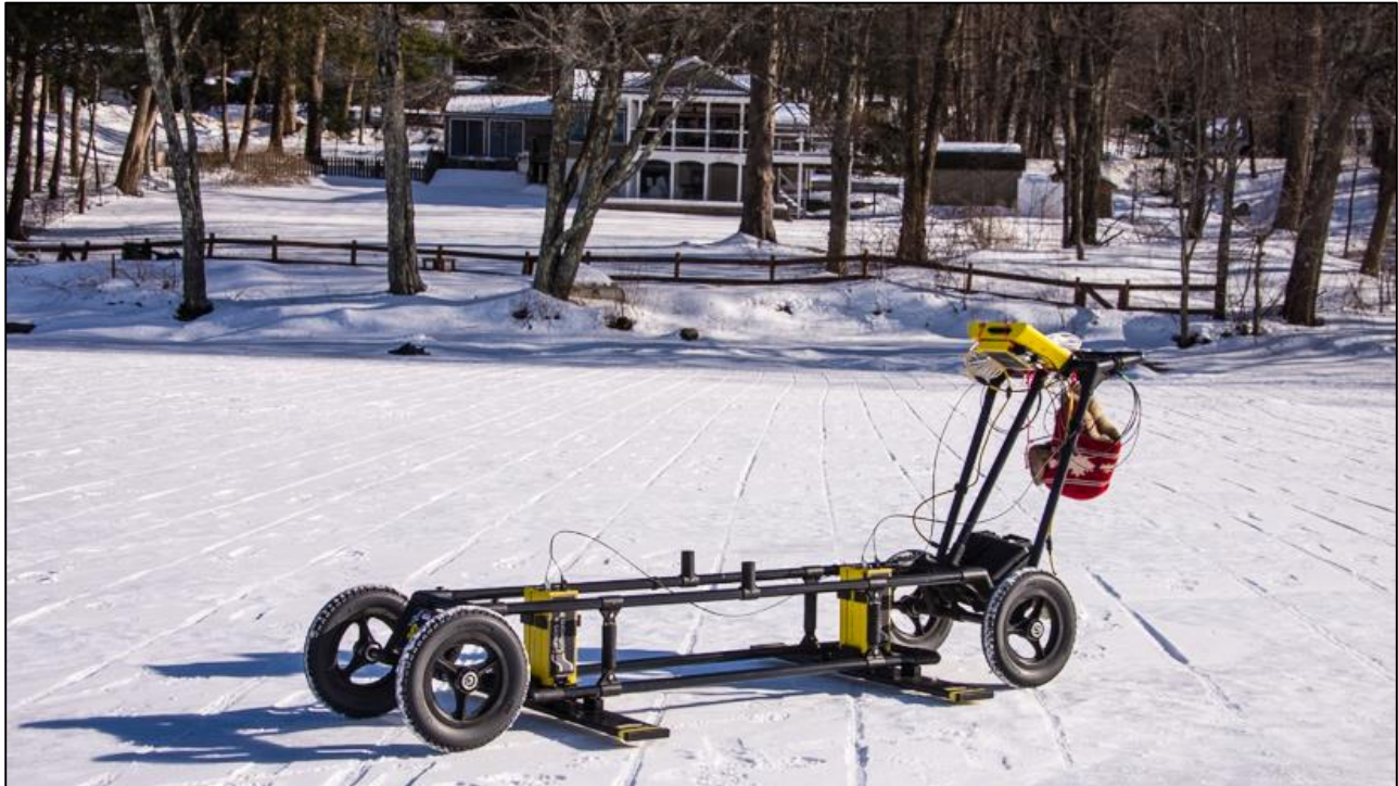
Figure 11. View to the SSE of the Pulse Ekko Pro GPR and smart cart at the time of data collection. Wheel lines visible in the snow indicate the direction of travel while collecting GPR data.
